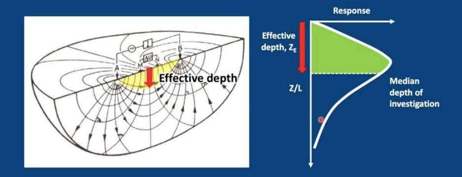
**EFFECTIVE DEPTH**  $(Z_E)$  = the interval within the subsurface of a homogeneous earth that contributes 50% of the measurement. Edwards (1977)
