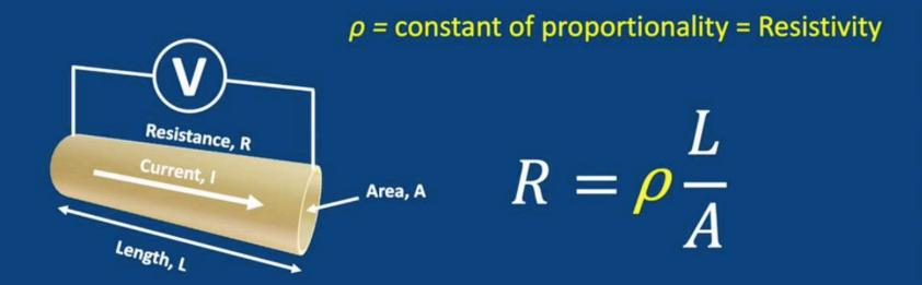
– Resistivity,  $\rho$  is a fundamental physical property of the metal in the wire
